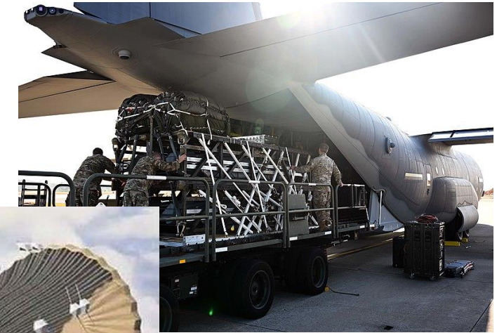
A Rapid Dragon module being loaded on a C-130 for airdrop.
